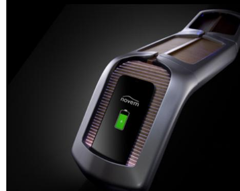
Centre console with sustainable lime wood panelling and integrated wireless charging application
